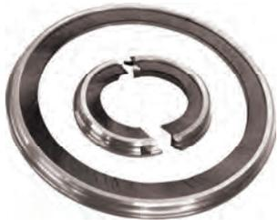
The Sentinel FBS is intended to be a drop-in replacement for a standard carbon ring seal. The brush serves as the primary shaft seal while a carbon element provides face sealing in the turbine’s casing. Users have found that by utilizing the FBS, the interval between seal replacement increased more than 3x to an average 3 to 4 year life span.
